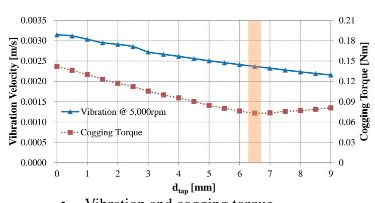
Vibration and cogging torque according to the center point of rotor. 0.0005 0.0004 0.0003 0.0002 0.0001 **Time Harmonics**
