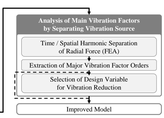
• Process of the vibration analysis using spatial harmonics and time harmonics of radial force density
