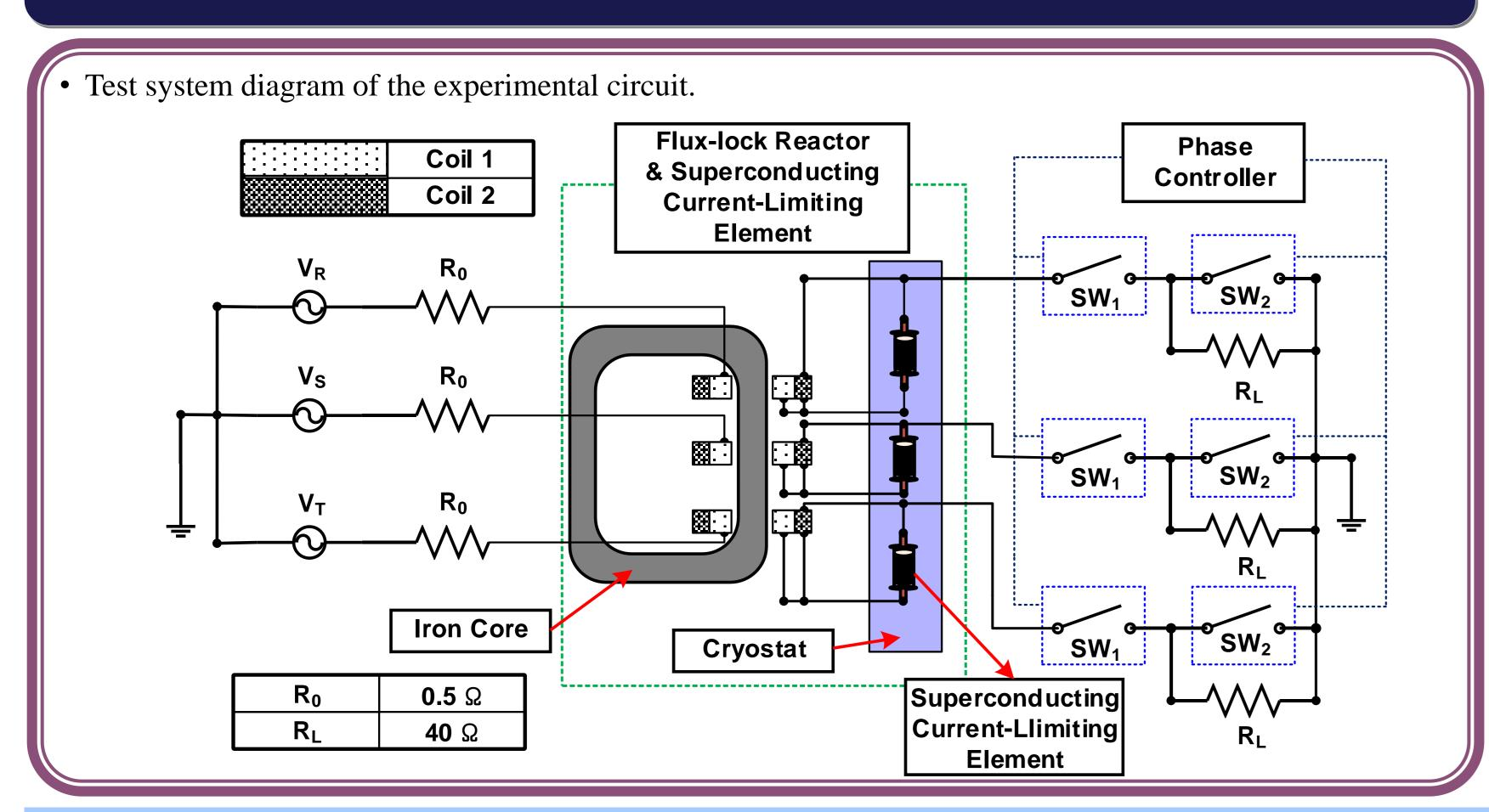
4. Structure and principle of operation of the model with the iron core and coil separated into three phase and the integrated model
