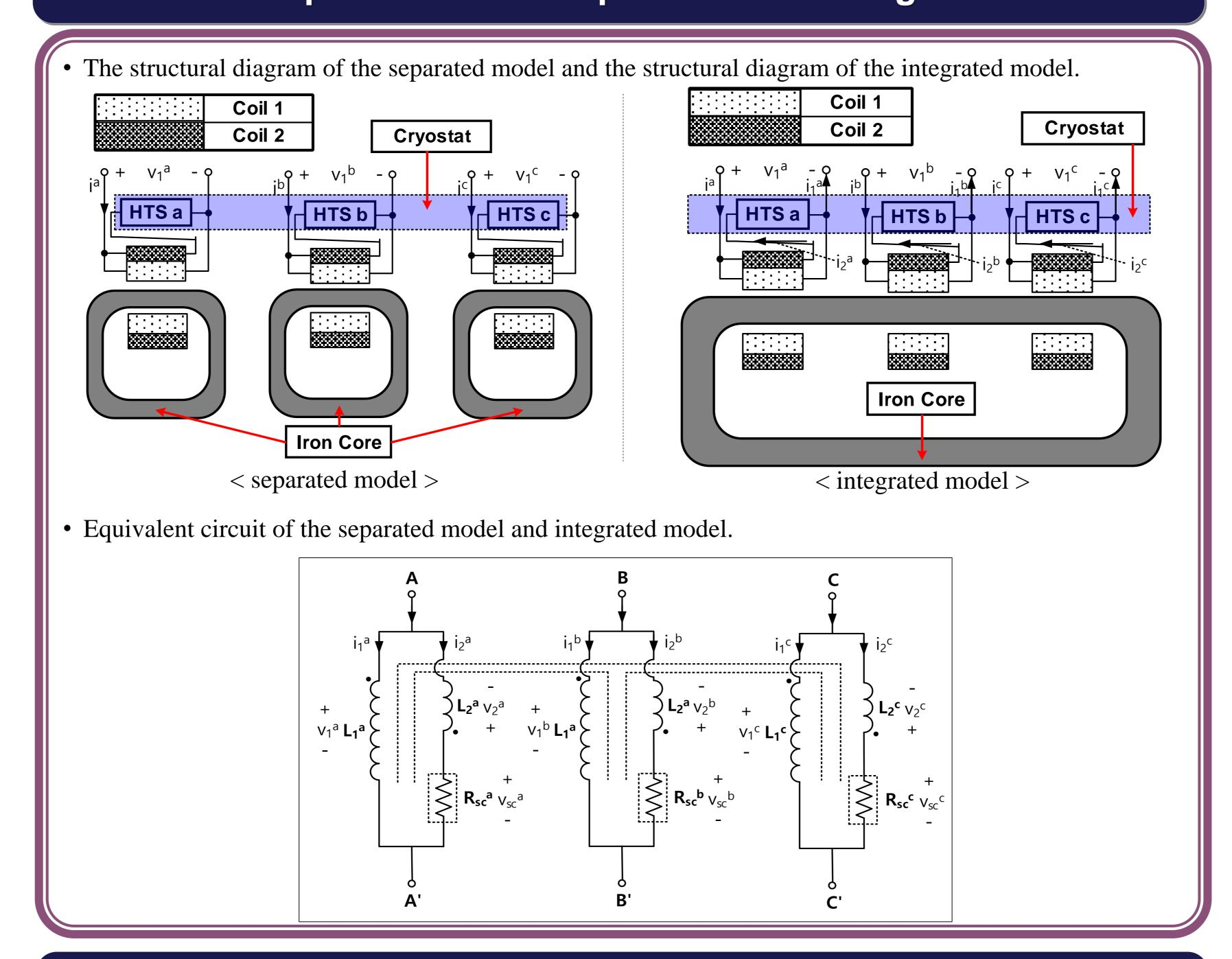
5. Analysis of current limiting characteristics of the integrated model of iron core and coil and of the model with separation thereof
