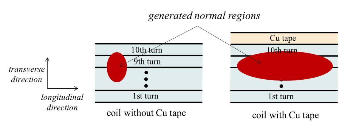
Schematic drawing of the predicted normal-state transition in both test coils with/without Cu tape
