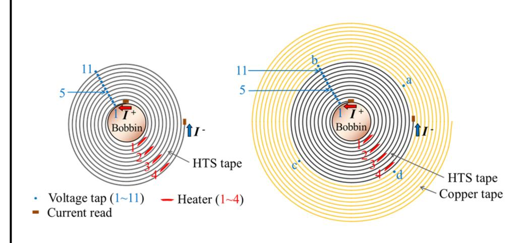
Schematic drawing of 10 turns NI test coils with/without a Cu protection ring
