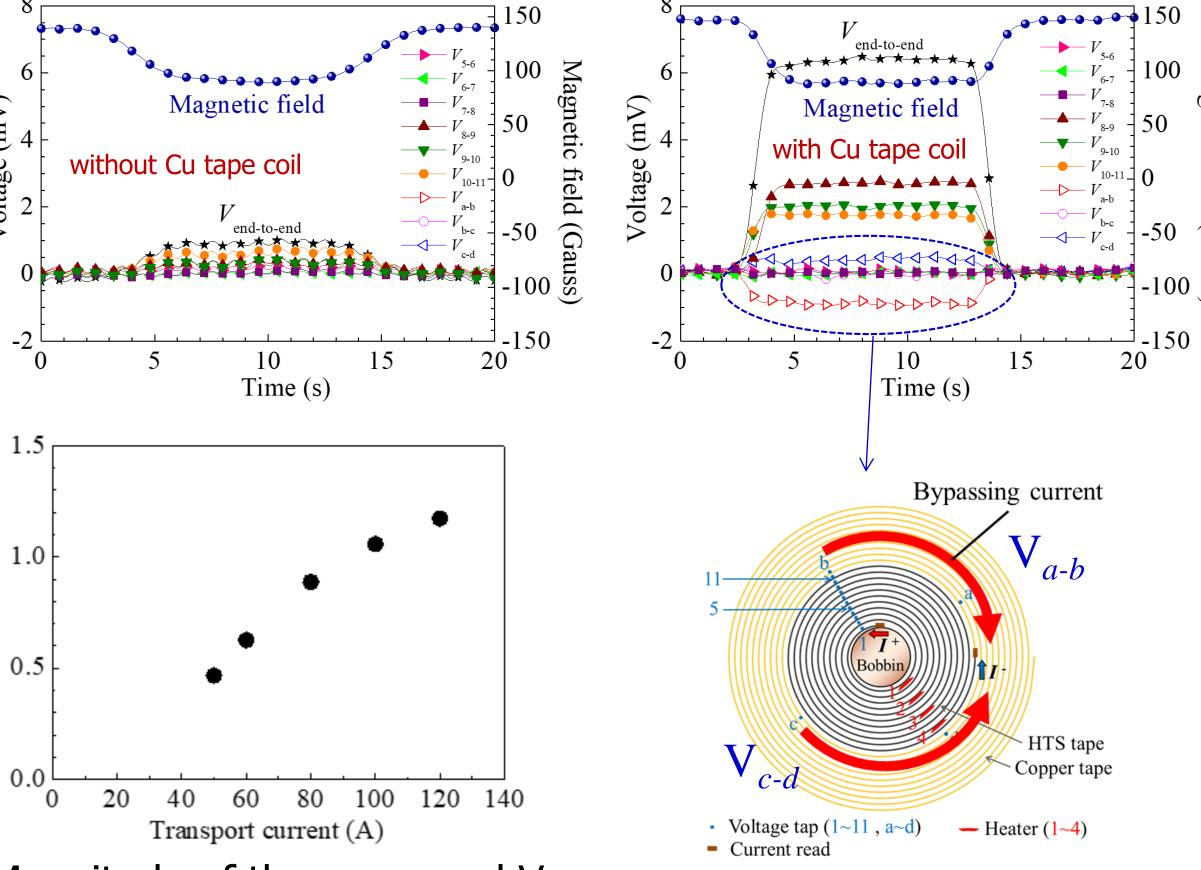
Magnitude of the measured V<sub>a-h</sub> (Heater4, 10 W input)
