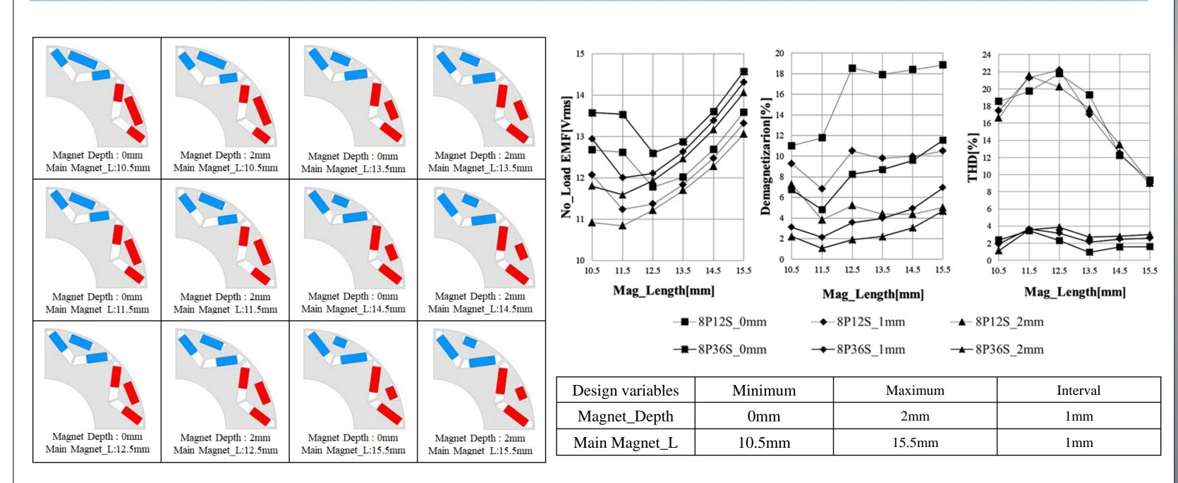
In the case of the Double Type, the magnet usage is the same and the length of the Sub magnet is reduced to have the same magnet usage as the length of the Main magnet increases. As the main magnet length increases, the back EMF and demagnetization increases above a certain size. The deeper the magnet insertion depth, the more the leakage magnetic flux was generated and the counter electromotive force was also reduced.
