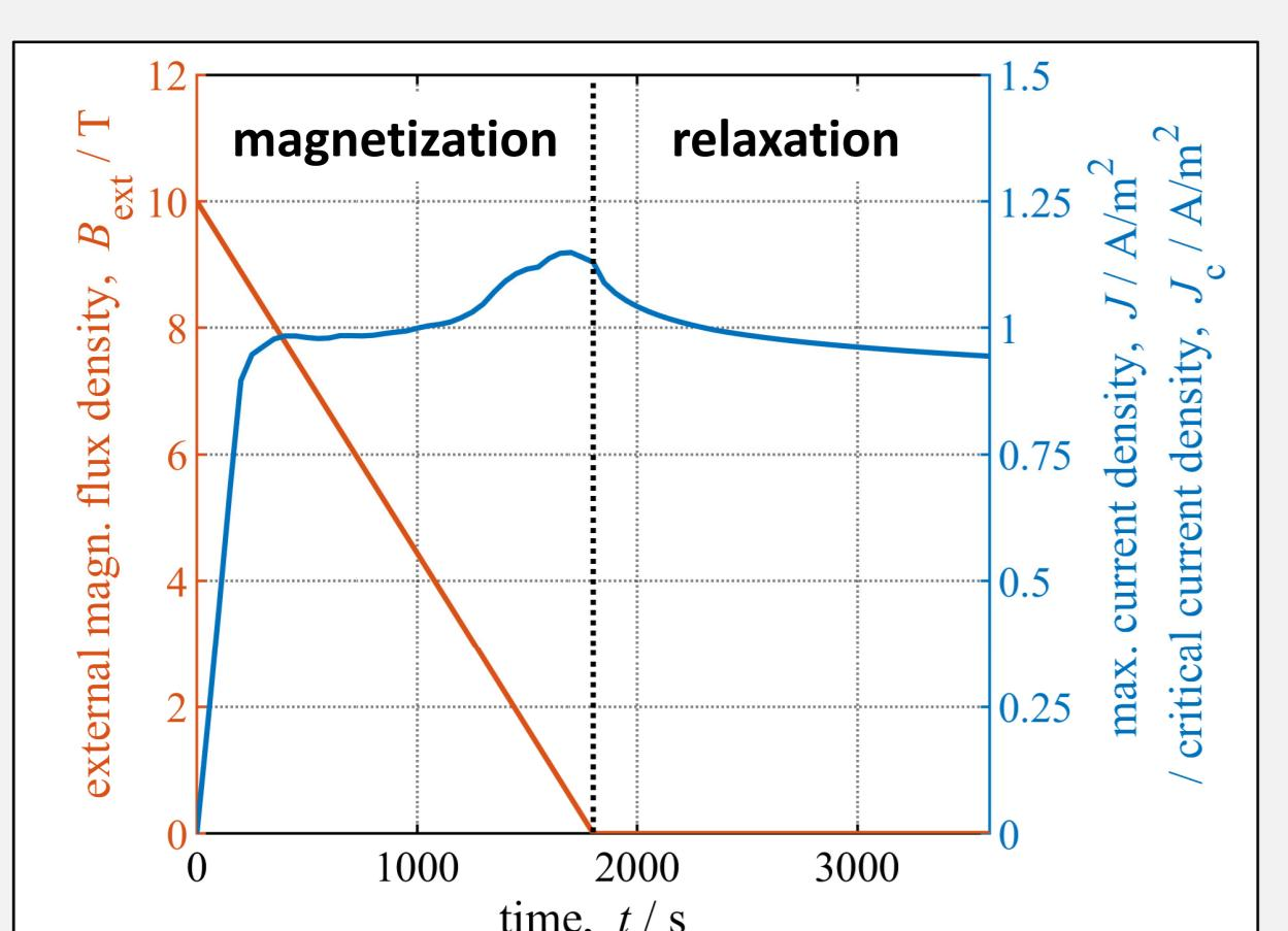
Trapping currents above the critical current density  $J_c$  is possible in the flux-creep model. This especially applies for short magnetization times.
