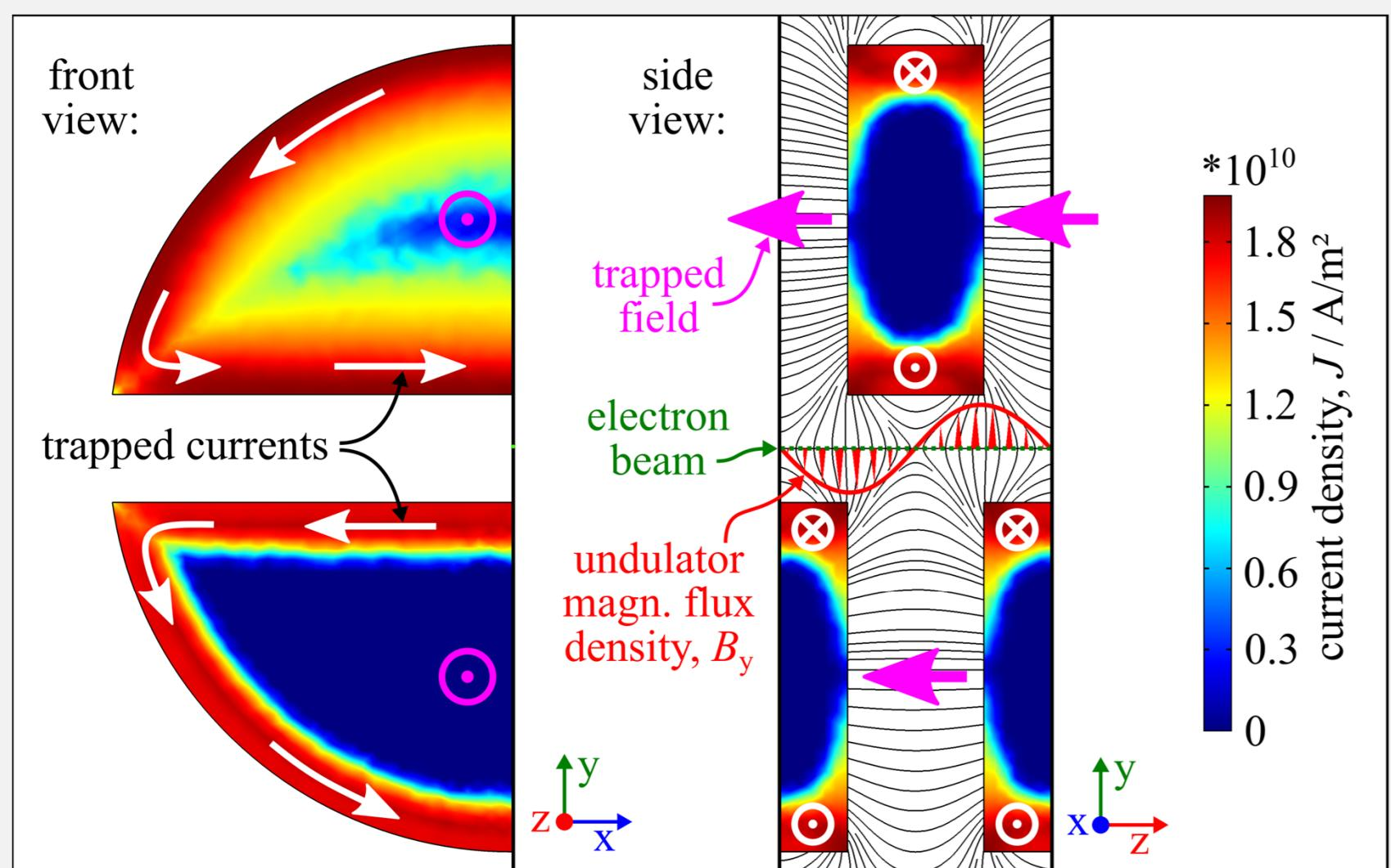
The undulator field,  $B_y$ , in the staggered array undulator is created by the stray components of the main trapped field traversing between the upper and lower row of ReBCO bulks
