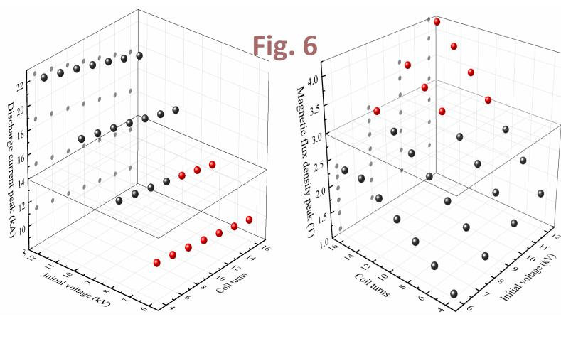
When initial voltage is 8 kV, number of coil turns is 16, a 3 T magnetizing field is generated with a temperature rise less than 100 K.
