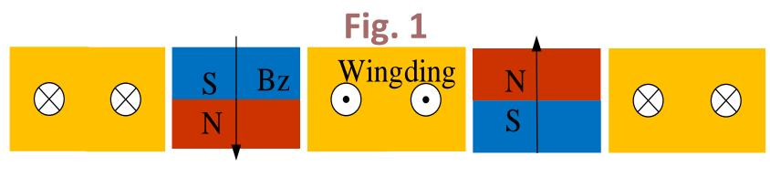
During the magnetization progress of the 900 kW SPM motor, the parts of the core close to the poles to be magnetized are locally saturated, resulting in asymmetry of magnetic circuits of the poles to be magnetized.
