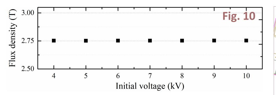
For the 900 kW motor, the stator windings barely have contribution to the magnetizing field
