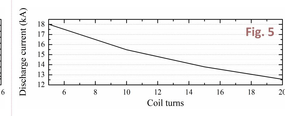
Parametric analysis of initial discharge voltage and number of coil turns
