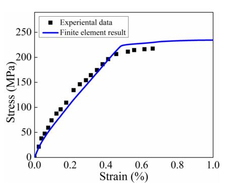
✓ The strain-stress curve of the single strand is in good agreement with the experimental data.
