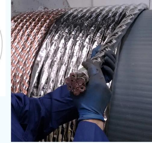
Thin spiral (0.5 mm thick strip): too large deformations during CICC compaction. It was 1 mm in 2015 High Field prototype.
