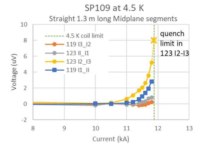
Voltage measured at 2 minute flattops for different current levels give the points in the V-I curves. The left figure shows all 4 straight mid plane segments in model SP107, the right figure the curve for SP109.
