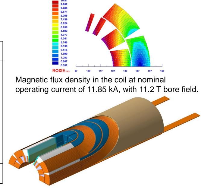
Image of the head of a coil, showing the impregnated coil part. The sliding pole is placed between the lightblue stainless steel pole shims.
