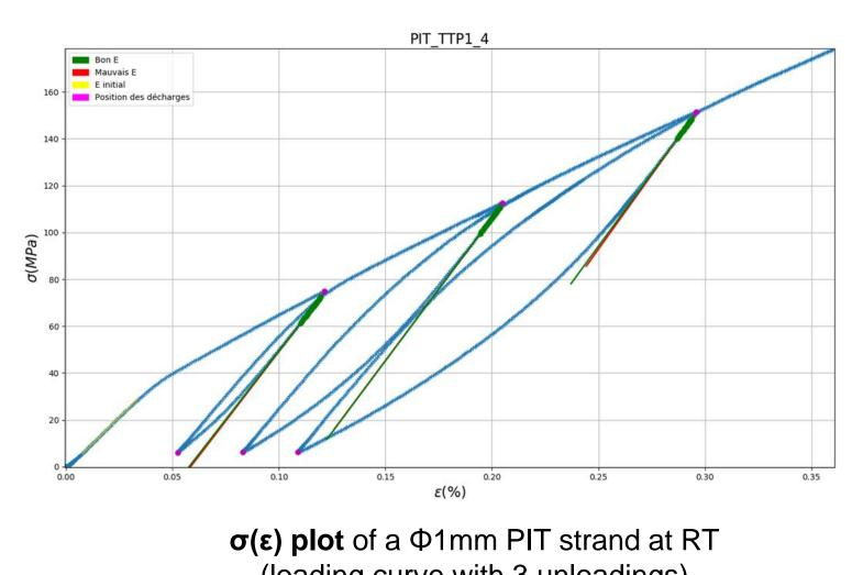
(loading curve with 3 unloadings) Scripted post-treatment locates unloadings and evaluates automatically the relevant slopes used for identification
