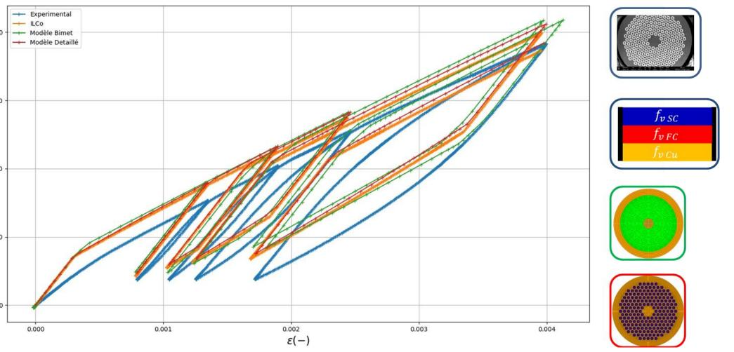
**Identification of the microstructure parameters** is performed using ILCO routine [4] by iteration on an analytical strand model based on volume fraction. Identification results are injected in 2 FEM strand models (detailed model / bi-material model) for comparison with experimental plot.
