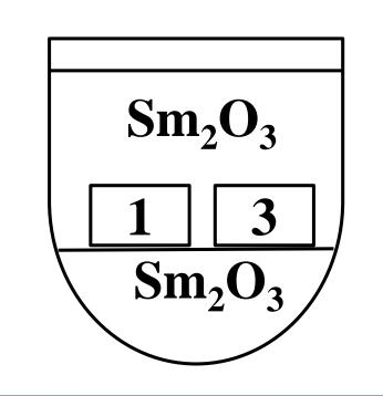
This is the figure of the 20 mm 1 and 3 specimen placed on top of and then covered with  $Sm_2O_{3.}$  The specimen must be covered on all sides with  $Sm_2O_{3.}$
