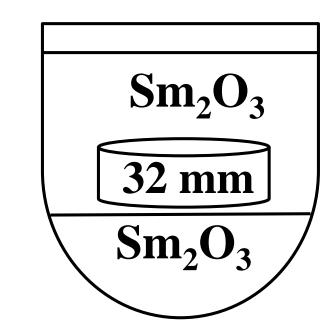
This is the figure of the 32 mm specimen placed on the top of and then covered with  $Sm_2O_3$ . The specimen must be covered on all sides with  $Sm_2O_3$ .
