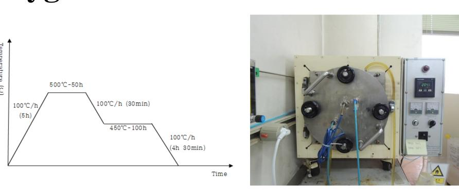
► Test the 32 mm specimen and the number 1 20 mm specimen using the following oxygen heat treatment conditions.
