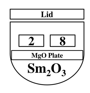
This is the figure of the number 2 and 8 20 mm specimens placed on top of the MgO plate which in turn is placed on the Sm<sub>2</sub>O<sub>3</sub>. After which is all covered with a lid and subjected to heat treatment. The specimens must not touch the Sm<sub>2</sub>O<sub>3</sub>.
