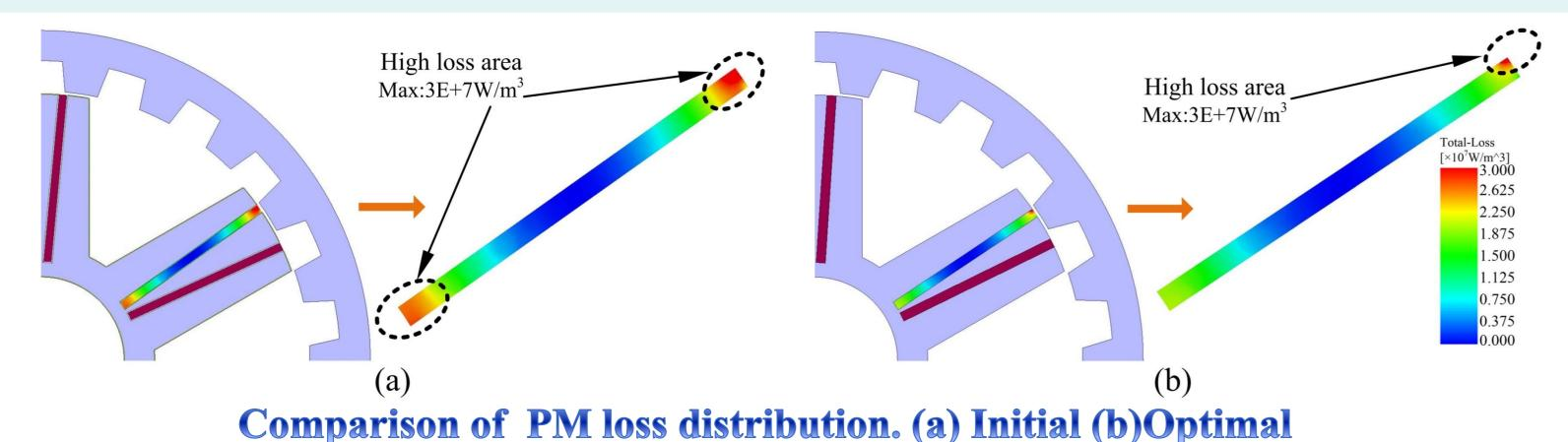
The high PM loss area of the optimal motor is almost eliminated completely, and low PM loss design is achieved.
