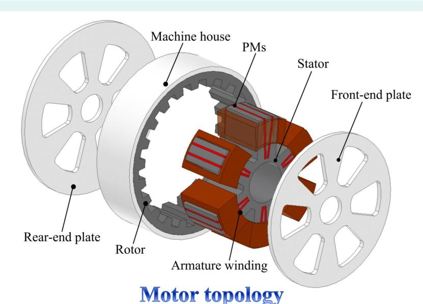
A V-shape out-rotor flux modulated permanent magnet motor is investigated in this paper.
