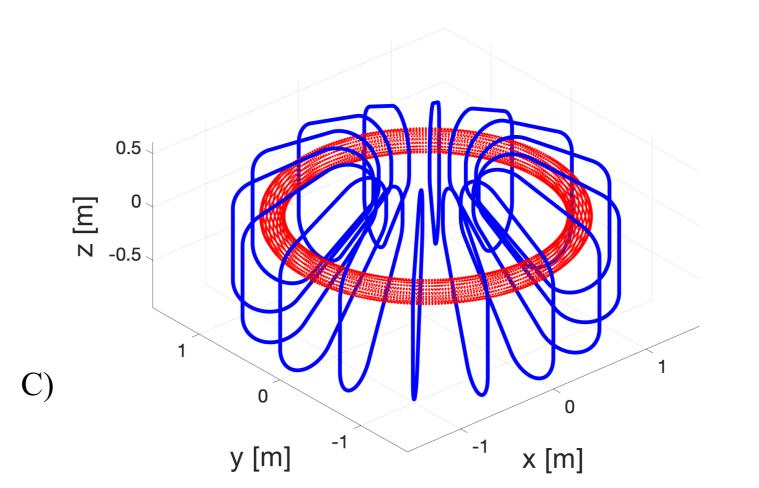
A fine discretization of each coil is required to reach a high computation accuracy.
