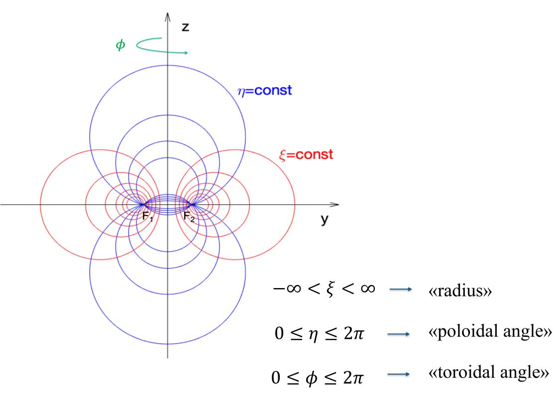
The procedure followed for the evaluation of the field harmonics is based on the Laplace equation\_solution for the magnetic scalar potential  $\psi$ , in toroidal coordinates.
