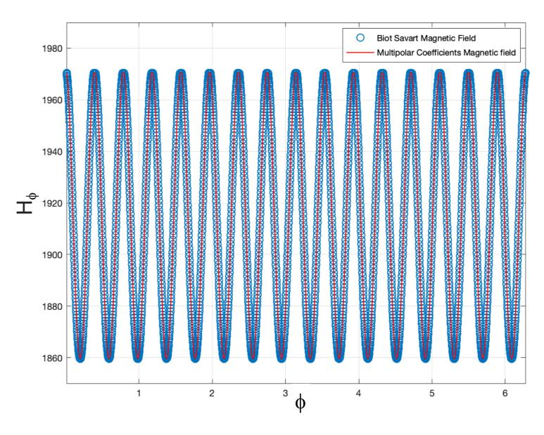
Magnetic field component  $H_{\phi}$  in Case A, at fixed  $\eta = 0.6$  rad; maximum relative error  $1.4 \times 10^{-5} \%$ .
