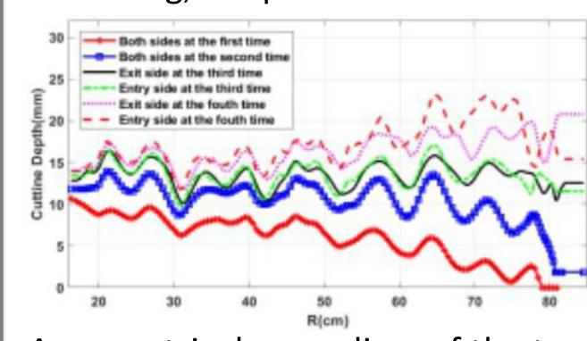
Asymmetrical amending of the two pole edges are introduced to adjust the local spiral angle and thus enhance the vertical tune. After two times of asymmetric amending, the vertical value reaches 0.15.
