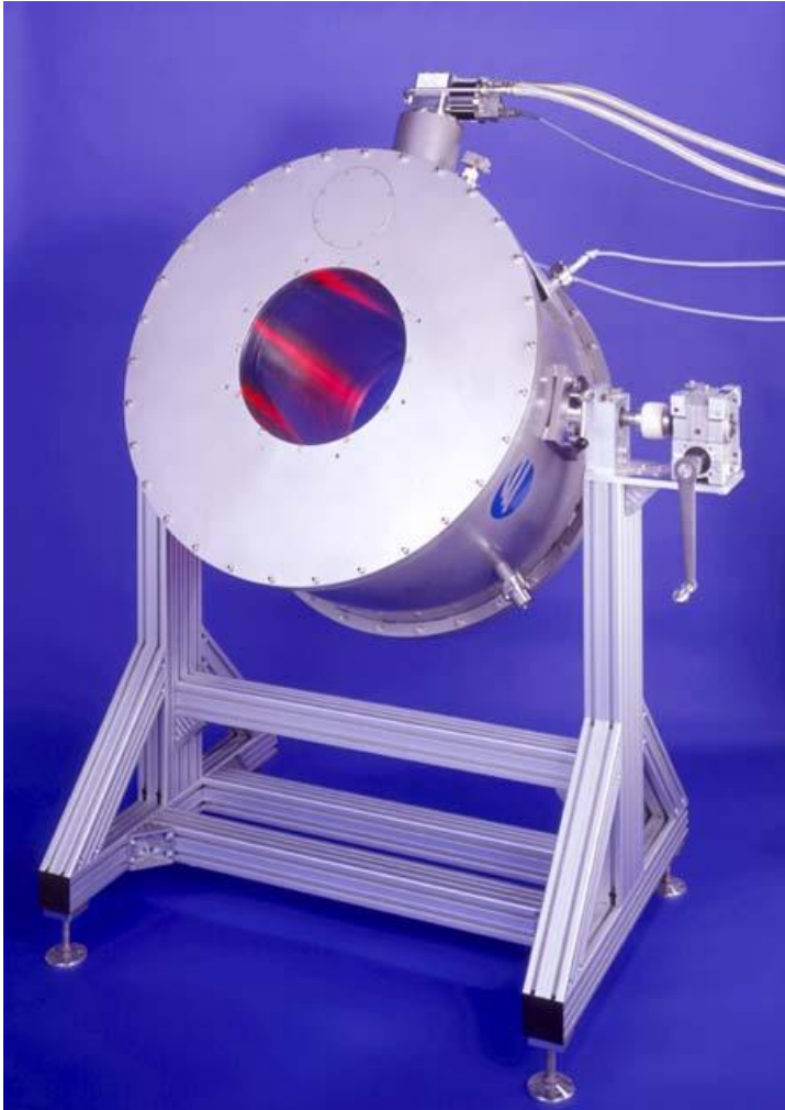
4 T magnet (Accel) cooled by Gifford-McMahon cooler
