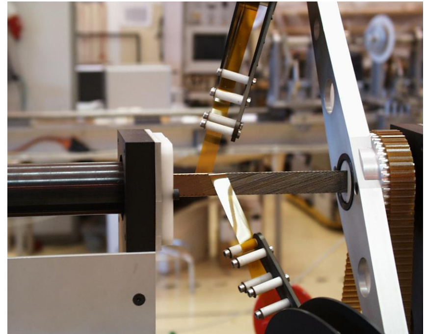
Cable insulation by double polyimide wrap
