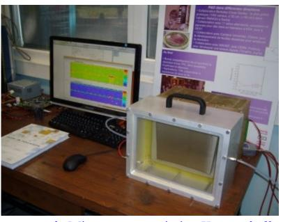
1726 pads Micromegas resistive Kapton bulk
