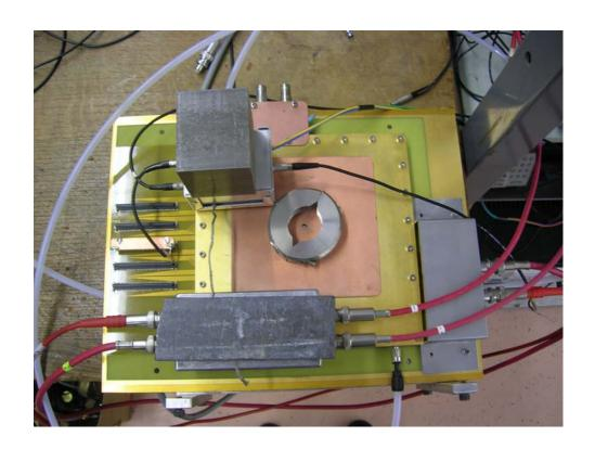
Measurements with <sup>55</sup>Fe / <sup>241</sup>Am and long integration time (1 μs)
