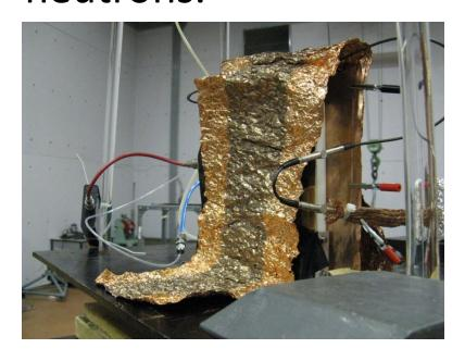
The chamber was completely covered with a copper foil in order to shield it from electromagnetic noise
