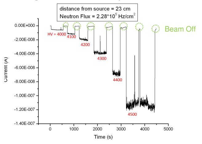
This is the "real-time" measurement: we were changing HV over time and measuring the anode current. We saw three current drops: we do not know if they are discharges or period during which the beam was off
