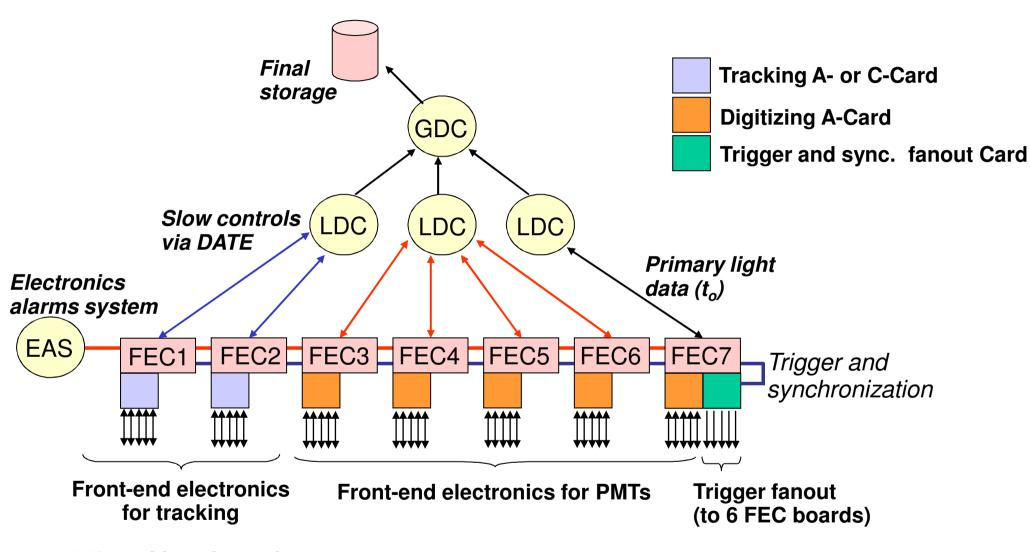
440 tracking channels 64 Energy ch (4 FE cards, 16ch/card) 14 FE cards (32ch/card) +(1-to-4) primary light channels
