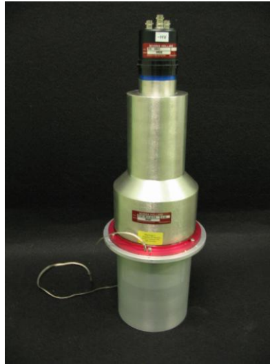
EJ-301 5"x5" Fast PMT Photonic XP4508
