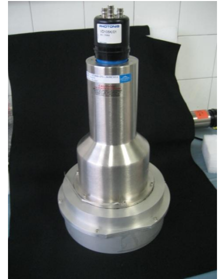
BC-501A 20x5cm Fast PMT Photonic XP4512
