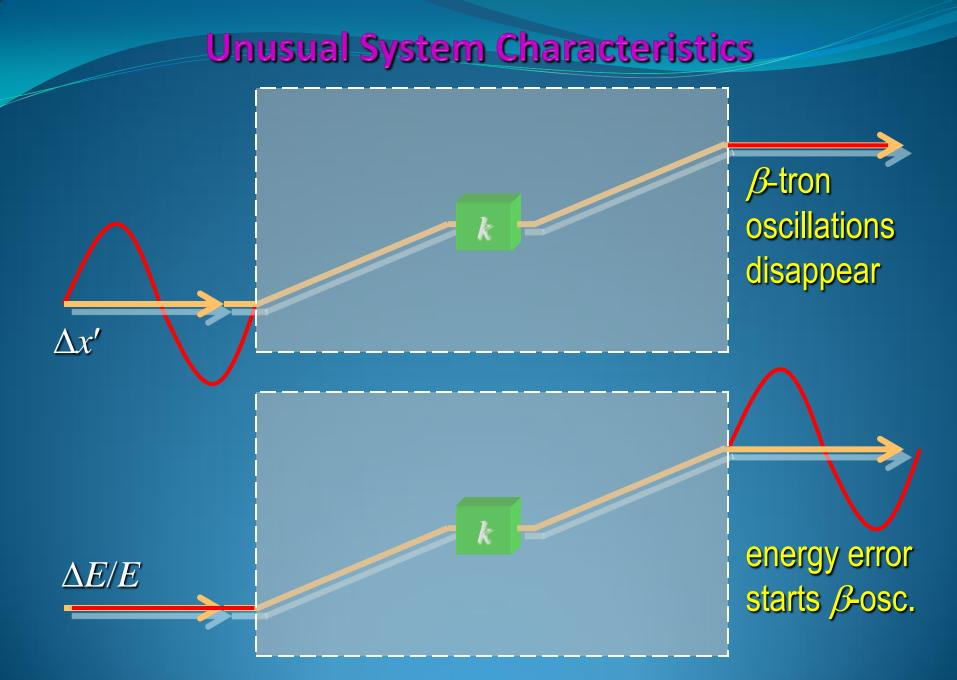
Need **extremely** stable energy (0.5×10<sup>-6</sup> rms jitter  $\Rightarrow$  10% x-beam size jitter)
