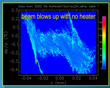
Final LCLS long. phase space at 14 GeV for initial modulation of 1% at  $\lambda_0$  = 15  $\mu{
