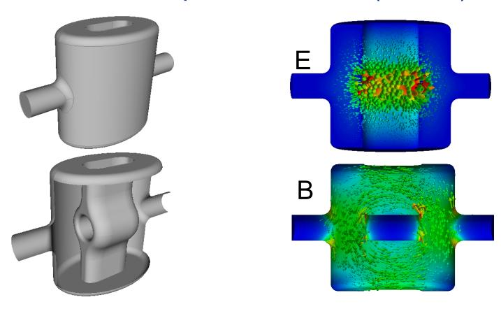
TE11-like mode - Frequency determined by longitudinal and vertical dimensions
