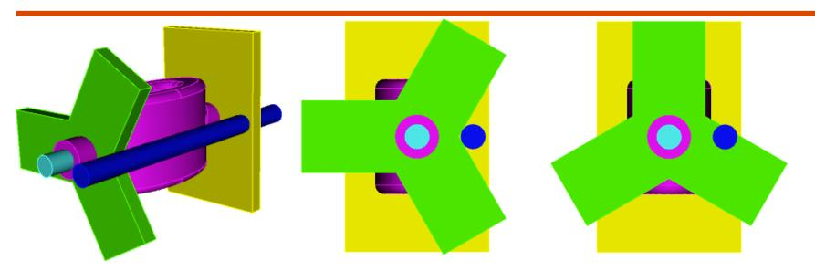
Waveguide couplers become large at low frequencies
