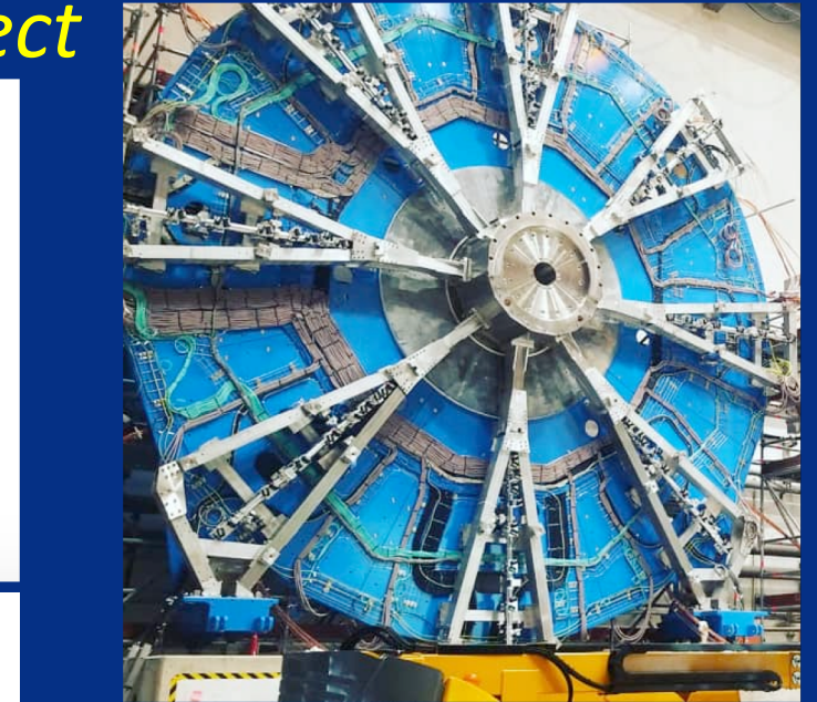
Mounting of services, small sector spokes (+ alignment bars) on support disk finished
