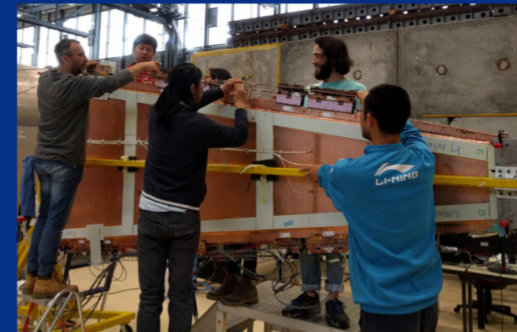
Mounting of services, small sector spokes (+ alignment bars) on support disk finished
