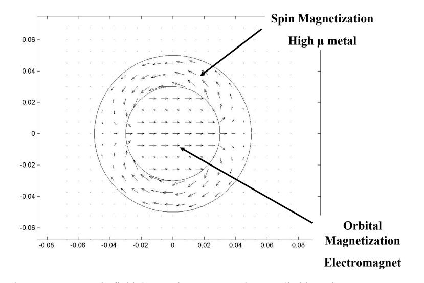
Outside spin source, magnetic field due to electromagnet is cancelled by spins
