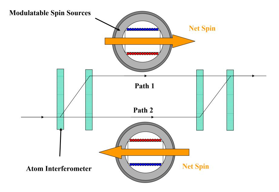
Axion signal can be nulled / combined / modulated as required
