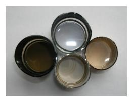
The irradiated and non irradiated samples are easily distinguishable. One can see that the HAMAMATSU glass @1.9 Mrad degraded by several %, which is significantly less than FEU-85 @1 Mrad. Generally, the glass degradation in our PMTs does not seem to be a problem.
