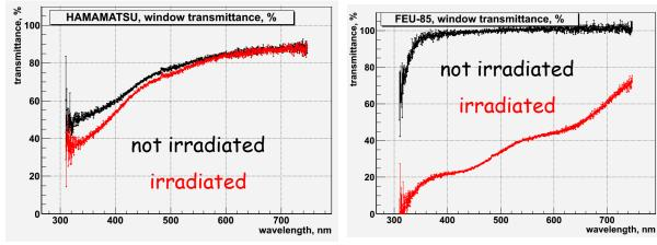
Not checked: PMT gain degradation at several hundred Coulomb
