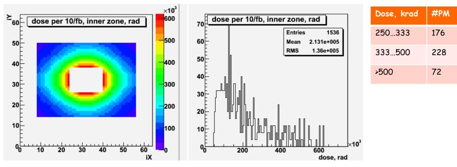
Assuming 4 years of operation at 10 /fb /year, we will have to perform replacement of irradiated CWs. Replacement of CW board on PM: an easy procedure taking ~ 10 minutes/board or less.
