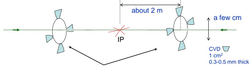
One Beam Conditions Monitor (BCM) on each side of IP:
