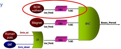
BCM protects against circulating beam failures, not against injection and extraction failures, though it will be ON during injection (for fast feedback).
