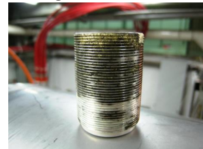
Contact erosion on Exit Box Replaced on 18 out of 30 generators installed
