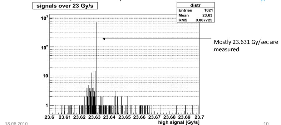
Restriction on LSA level (max. thresholds): 250 counts \* 1024 = 256000 BITS = 23.168 Gy/sec
