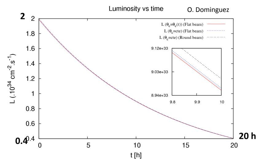
Time evolution of the HE-LHC luminosity, for both flat and round beams, including emittance variation with controlled blow up and proton burn off. Curves with constant or varying crossing angle lie on top of each other if the beam-beam tune shift is kept constant as assumed here.
