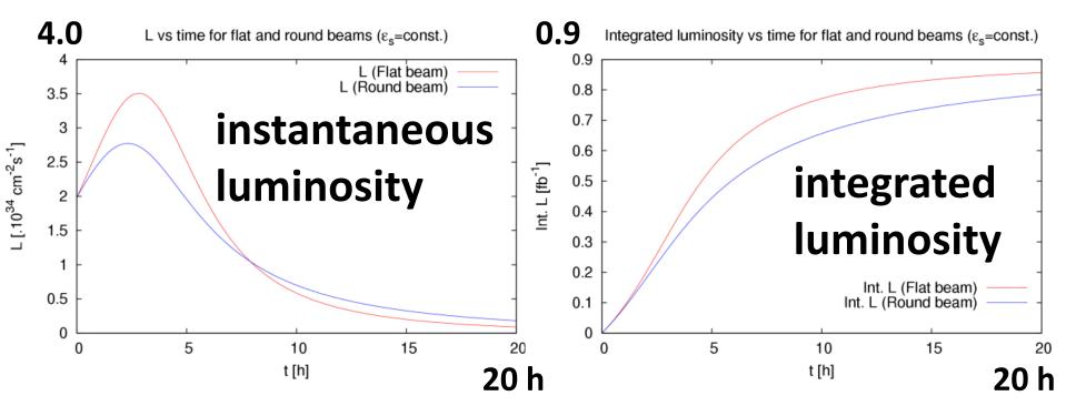
Time evolution of the HE-LHC instantaneous (left) and integrated luminosity (right), for both flat and round beams, including SR emittance shrinkage without controlled transverse blow up and including proton burn off.
