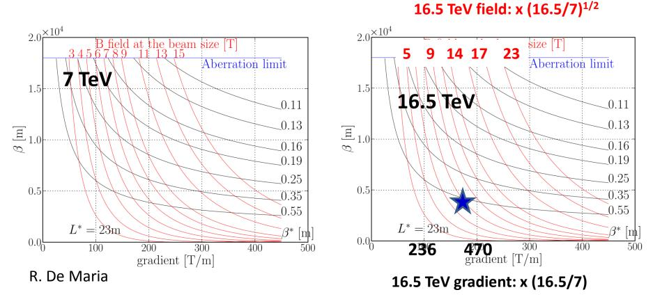
for example:  $\beta^*=0.55$  m, 400 T/m,  $\beta_{peak}$ ~4 km,  $\gamma\epsilon=2.64$  µm, full aperture ~26 mm
