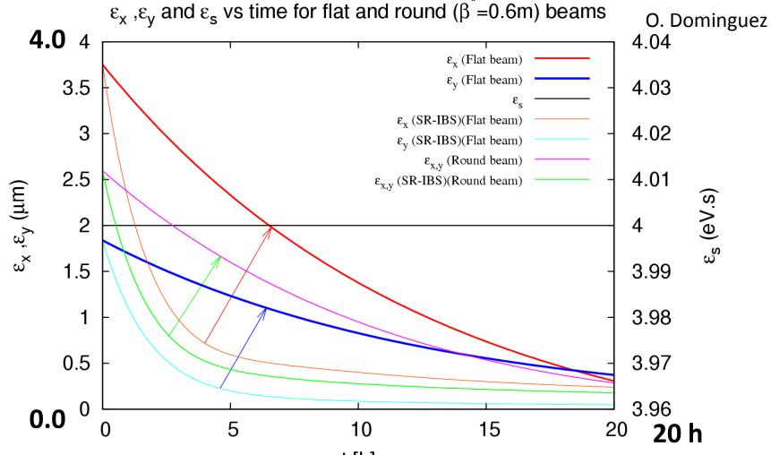
t [h] Evolution of the HE-LHC emittances, for flat and round beams, during a physics store with controlled blow up and constant longitudinal emittance of 4 eVs plus constant crossing angle (the thicker lines on the top), and the natural transverse emittance evolution due to radiation damping and IBS only (the thinner lines at the bottom) – still for constant longitudinal emittance and constant crossing angle –, which might lead to an excessive tune shift.
