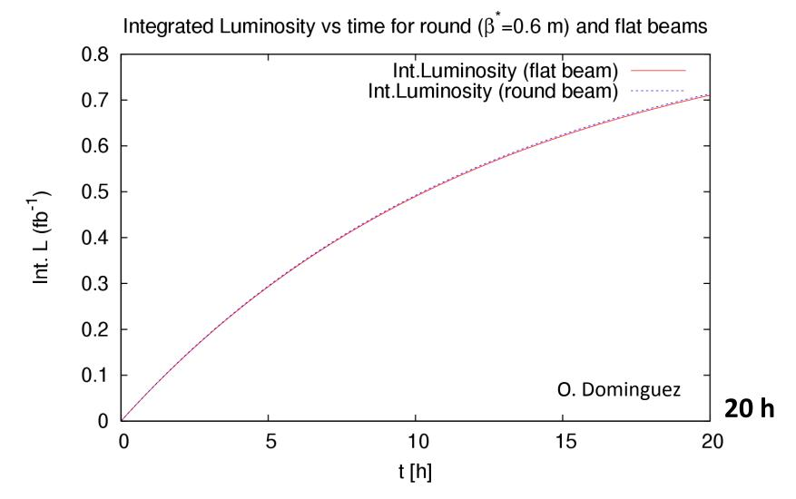
Time evolution of the HE-LHC integrated luminosity, for both flat and round beams, during a physics store including emittance variation with controlled blow up and proton burn off.
