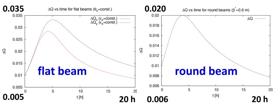
Time evolution of the HE-LHC tune shifts, for flat (left) and round beams (right), during a physics store including SR emittance shrinkage **without** controlled transverse blow up, and including proton burn off.
