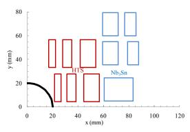
Figure 5: Block lay out of the coil proposed in [11] (one quarter of one aperture shown).
