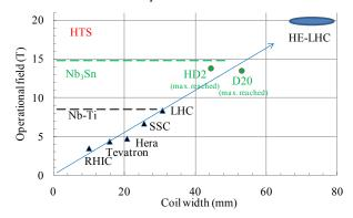
Figure 2: Operational field versus coil width in Nb-Ti accelerator magnets. For Nb<sub>3</sub>Sn models the maximum reached field is given. The straight line fit has a slope consistent with  $j_0=400 \text{ A/mm}^2$ .
