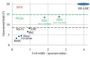
Figure 8: Operational field versus ratio coil width/aperture radius in Nb-Ti accelerator magnets. For Nb<sub>3</sub>Sn models the maximum reached field is given.
