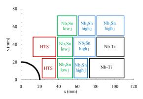
Figure 4: Block lay out of the coil (one quarter of one aperture only is shown).
