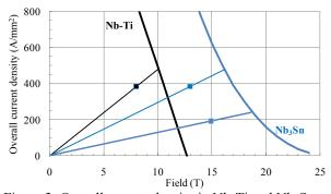
Figure 3: Overall current density in Nb-Ti and Nb<sub>3</sub>Sn (curves), loadlines (straight lines) and operational points.
