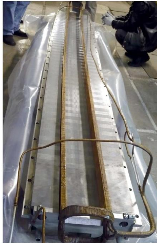
Figure 16 Top view of SIS100 curved magnet coil inserted into lower part of iron yoke.
