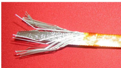
FIG.5: The 36 strand Rutherford cable. In between the strands one can see the thin stainless steel core used for depressing the inter-strand coupling currents.
