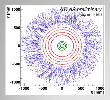
Pixel Detector: 3 barrel layers, 2 x 3 end-cap discs  $\sigma_{r\phi} \sim 10 \ \mu m$ ,  $\sigma_z \sim 115 \ \mu m$ Silicon Strip Detector (SCT) 4 barrel layers, 2 x 9 end-cap discs  $\sigma_{r\phi} \sim 17 \ \mu m$ ,  $\sigma_z \sim 580 \ \mu m$ Transition Radiation Tracker(TRT) 73 barrel straw layers, 2x160 end-cap radial straw discs  $\sigma_{r\phi} \sim 130 \ \mu m$
