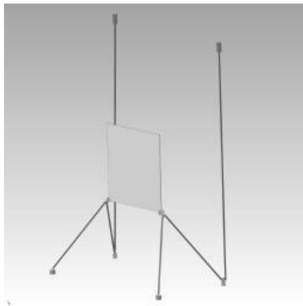
Figure 8: Mooring system (not to scale, simplified); note the bifilar suspension; the upper mooring system which completes the stabilization of the structure, is not illustrated.
