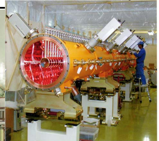
Inside of Drift Tube Linac
