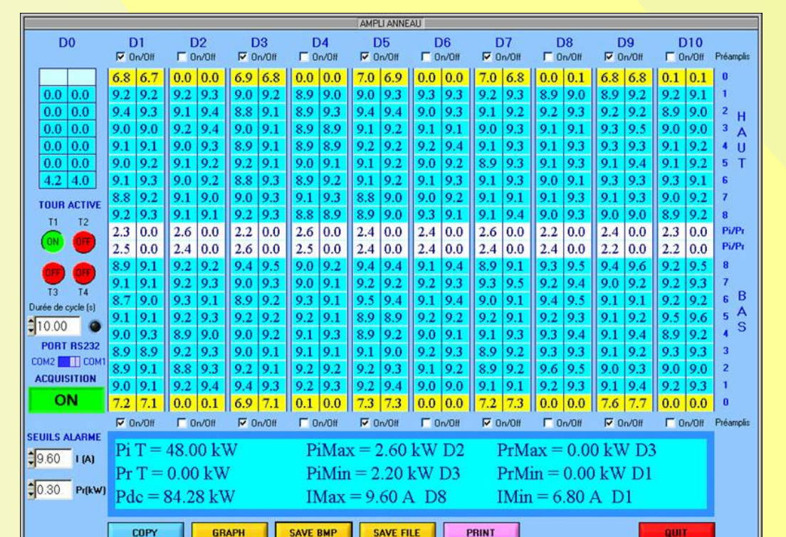
"50 kW tower" control display ( transistor currents, Pi & Pr )
