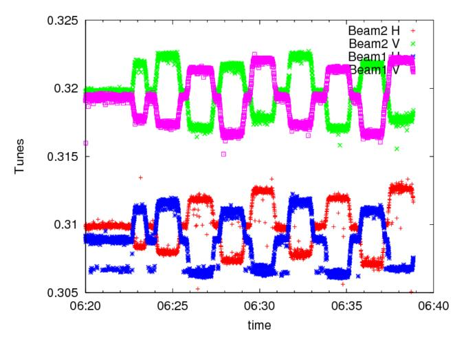
$\beta^*$  is calculated from the amplitude of the tune modulation when changing the gradient of triplet quadrupoles.
