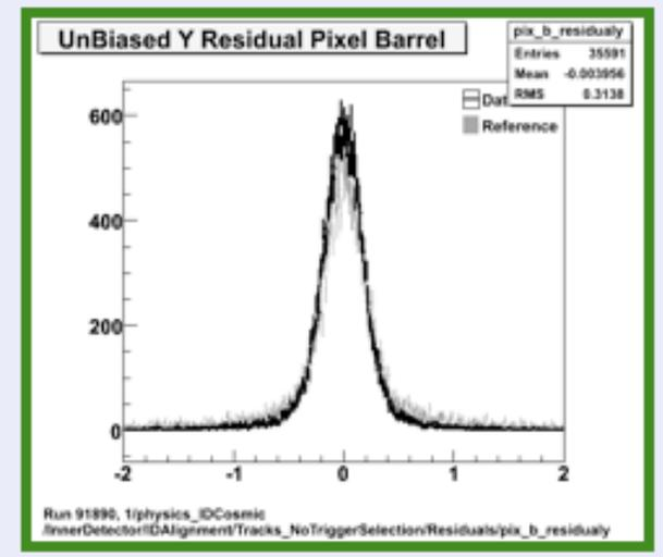
Colour of outer box of plot is indication of the DQ (from automatic comparisons)
