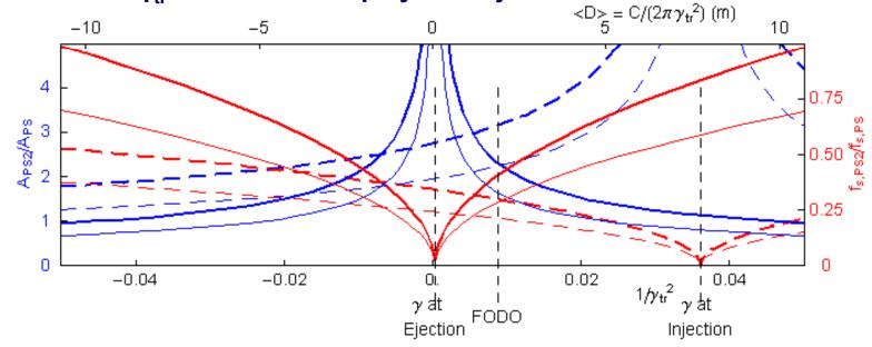
Acceptance (blue) and adiabaticity (red) ratios PS2/PS at injection (dashed) and ejection (solid)
