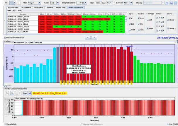
Figure 5: Post mortem analysis of dumping 32 bunches on the upper TDI jaw in P2.
