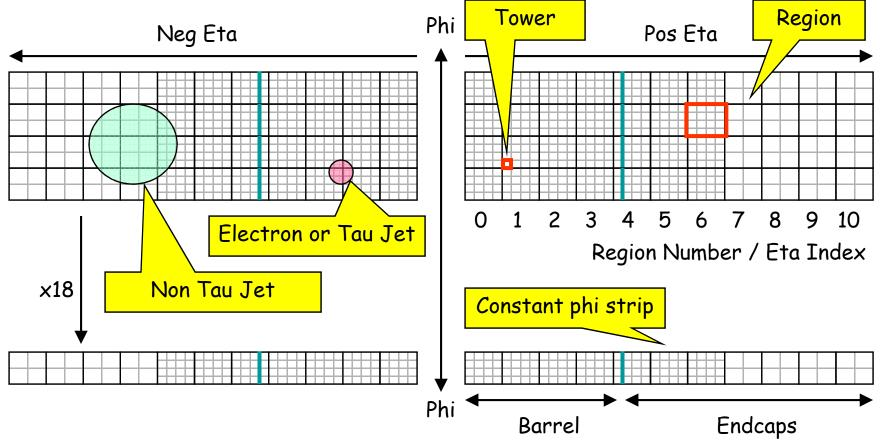
Data per tower, per bx ECAL: 8bits energy + FGV (FineGrainVeto) HCAL: 8bits energy + MIP (MinIonisingParticle) Geometry & link capacity
