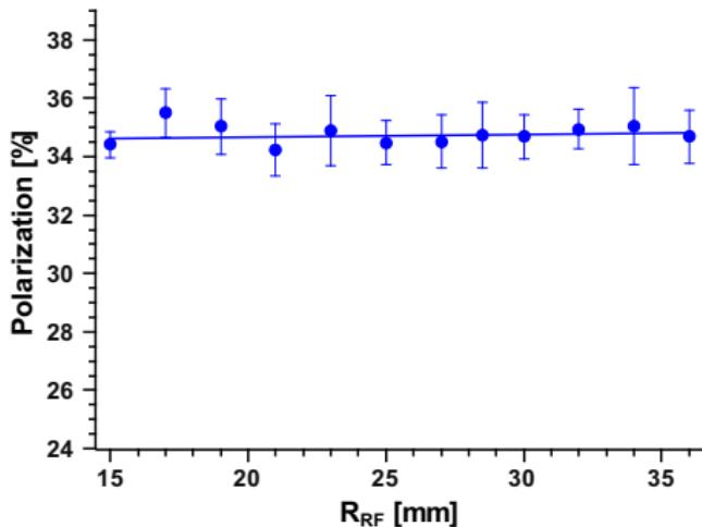
Optimal aperture of RF cavities is  $27 \div 29$  mm
