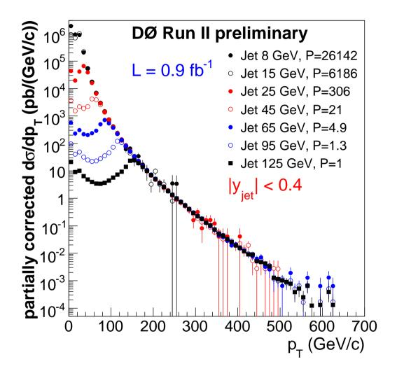
• due to steeply falling spectrum, the measurement of jet production is extremely sensitive to the precision of jet energy calibration
