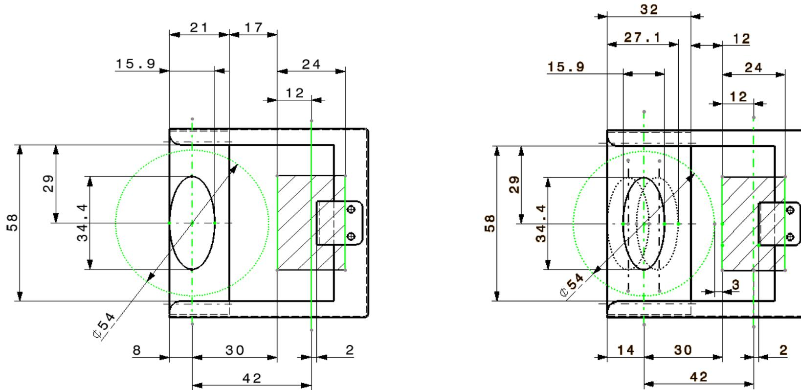
Estimated beam size on the foil for zero dispersion (left) and matched (-1.4 m) dispersion (right) at injection point. PSB beam envelope ( $\varnothing 54$ mm) during injection is also shown. (L4-T-EP-0005, EDMS 1108941)
