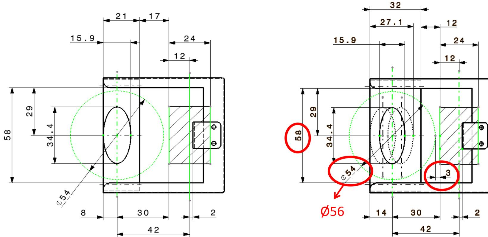
Estimated beam size on the foil for zero dispersion (left) and matched (-1.4 m) dispersion (right) at injection point. PSB beam envelope ( $\text{Ø}56\text{mm}$ ) during injection is also shown. (L4-T-EP-0005, EDMS 1108941)
