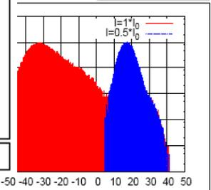
( MDX adjusted for  $\sim 10$  cm screen image:  $B \approx 20\text{mT}$ ,  $\theta_{\min} \sim 1^\circ$ ,  $\theta_{\max} \sim 5^\circ$  )
