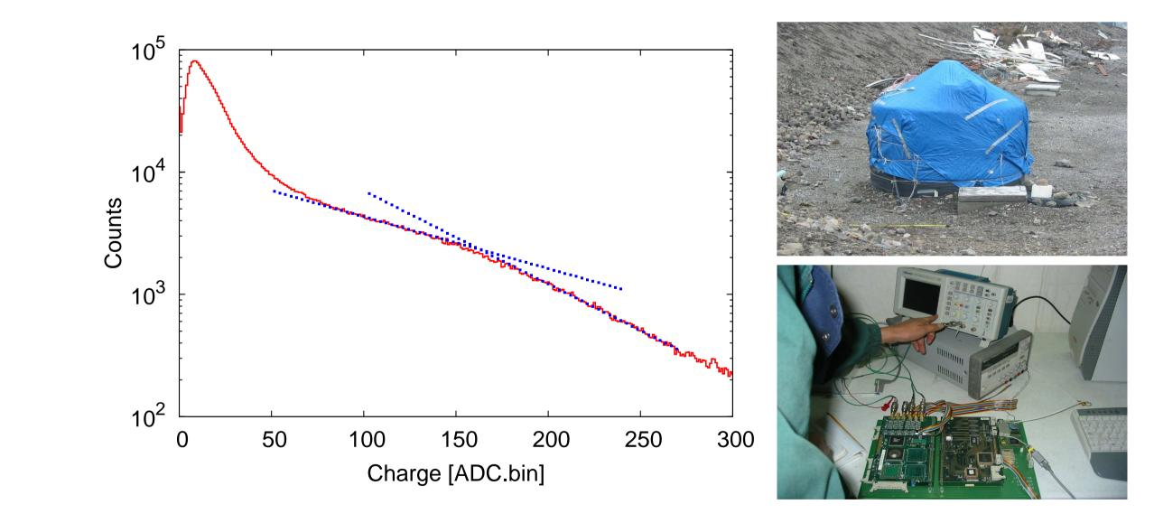
Three  $4 \text{ m}^2$  and two  $1 \text{ m}^2$  WCD are in operation at Sierra Negra. They are connected to a prototype acquisition board of the Pierre Auger Observatory running LAGO specific software. Calibration is done with the muon "shoulder" as shown on the plot above.
