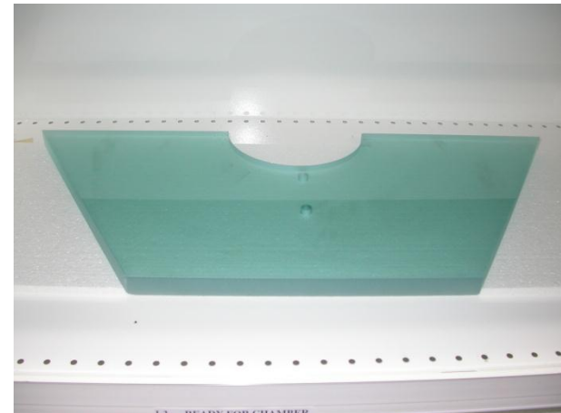
One of the hexagonal mirrors before aluminization.
