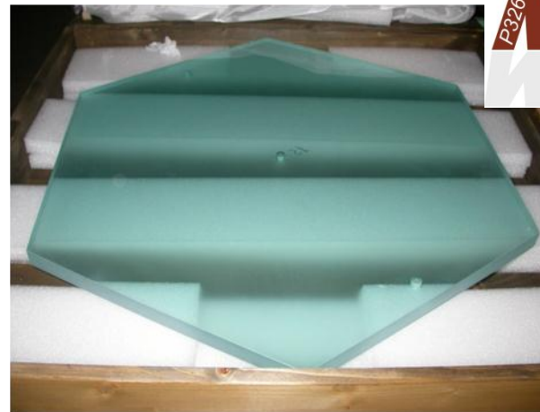
One of the hexagonal mirrors before aluminization.
