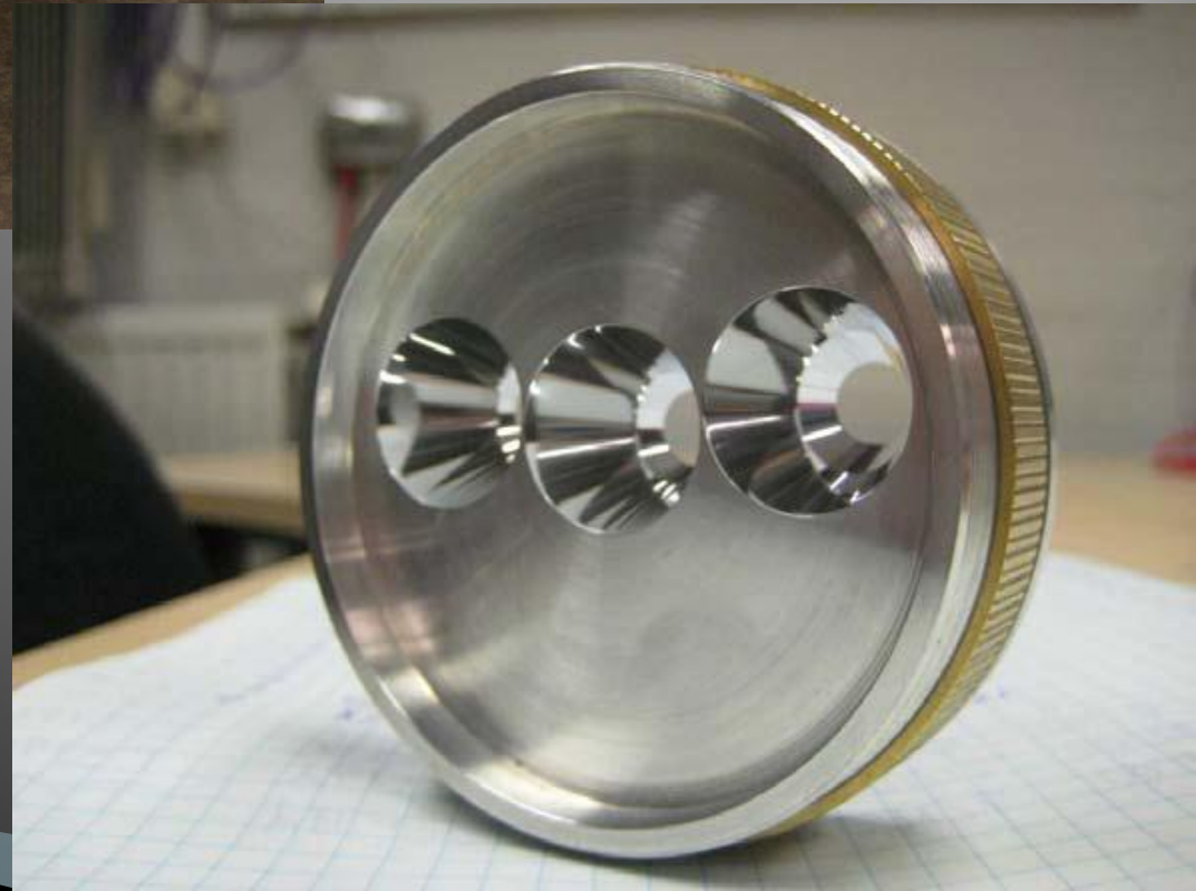
Aluminum light-guide (prototype) obtained by electric discharge machining in Liverpool
