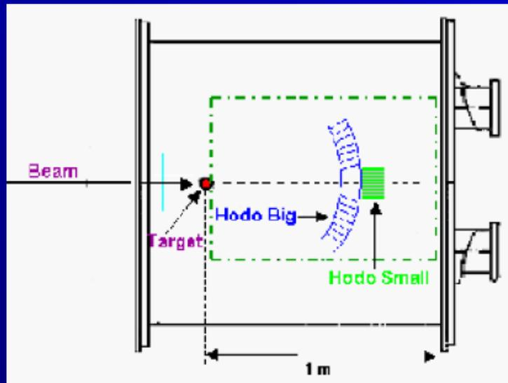
Schematic view of the scattering chamber with the beam entrance, target and experimental apparatus
