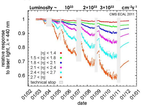
ECAL Barrel: crystals qualified for <6% loss under 0.15 Gy/h
