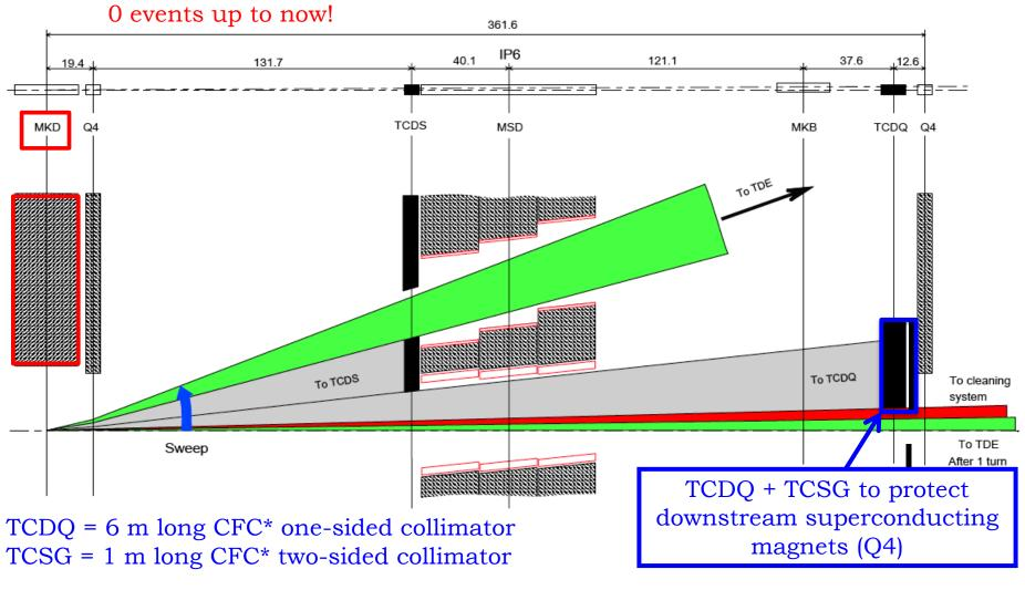
\*CFC = carbon fibre compound
