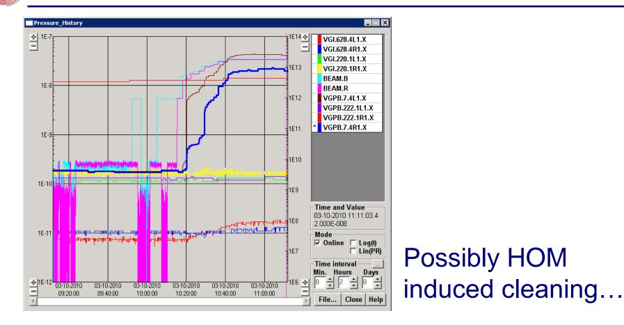
Inner Triplet left 1 (VGPB.7.4L1.X): Start pressure before filling: 1.8x10<sup>-10</sup>mbar End pressure after filling: **4.3x10<sup>-8</sup>mbar**
